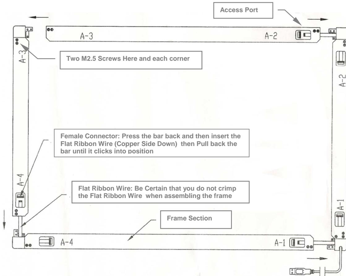
**Step Four:** In the access Ports that do not have a Flat Ribbon Wire already present, identify the female connector and notice a flat bar. This bar must be in the Open position to accept the Flat Ribbon Wire from the matching frame section. Using a small flat blade screwdriver, gently push the bar back into the open position if it is not already in the open position. It will be loosely held if open.
